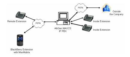
Like a remote extension, the BlackBerry running MaxMobile serves as an office extension, making and receiving calls through the PSTN (public switched telephone network) to and from your company's MAXCS system. You can call company extensions (both inside and remote extensions) just by dialing the extension number. Your calls to destinations outside the company can go through the MAXCS system, as illustrated in the previous figure, if you so choose.
